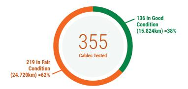
The majority of the cables Elexicon selected for testing were direct-buried residential cables from the 1970's and 1980's. With the majority of the cables being 40+ years old, they had theoretically reached the end of their nominal life expectancy. However, CableQ's Non-Destructive Cable Testing provided Elexicon with a health score for the cables, demonstrating that this was not the case.
